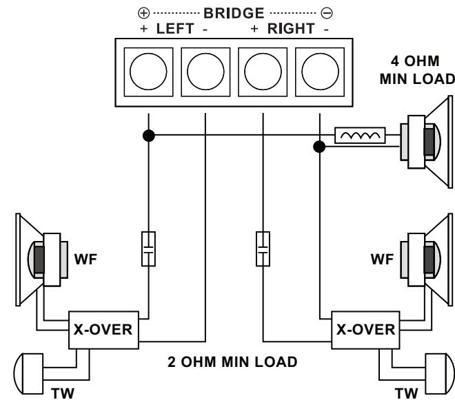
A 3-Way hookup requires a coil on the woofer and capacitors on the highs to act as a crossover and maintain correct impedance. Consult the speaker manufacturer for correct cap and coil values.
