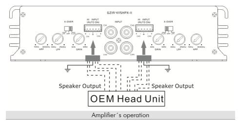
The amplifier will turn and off automatically, if the connections have been made correctly.
